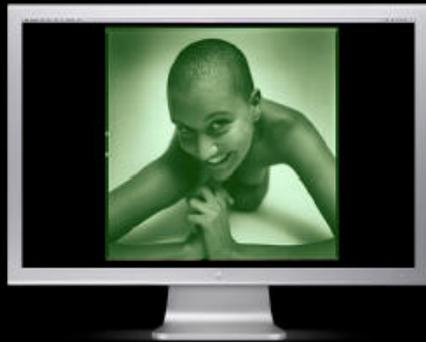
Same file displayed on an uncalibrated monitor resulting in a green cast
